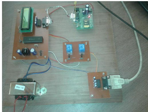
Figure 8 RF design for server unit
