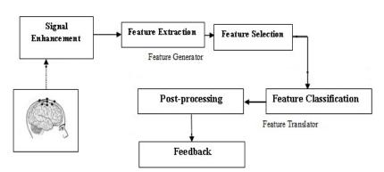
Fig 1: General model of EEG based BCI system
