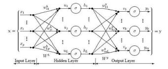
Fig 3: Three layer Perceptron network
