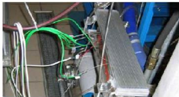
Fig. 2: Thermoelectric generator mounted on exhaust system.
