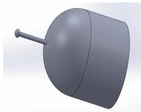
Fig. 6. Spherical Spike with L/D Ratio Of 1.0
