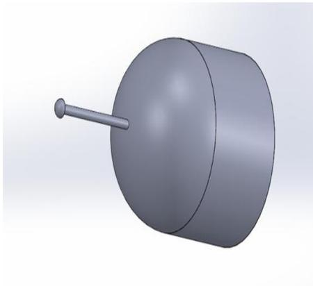
Fig. 7. Spherical Spike with L/D Ratio Of 1.5
