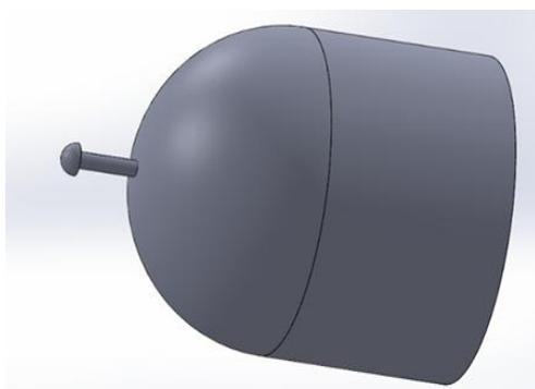
Fig. 5. Spherical Spike with L/D Ratio Of 0.5
