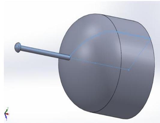
Fig. 8. Spherical Spike with L/D Ratio Of 2.
