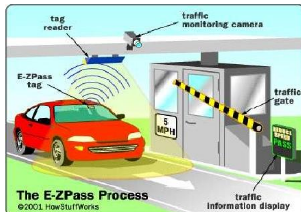
Fig.: Electronic Toll Collection System
