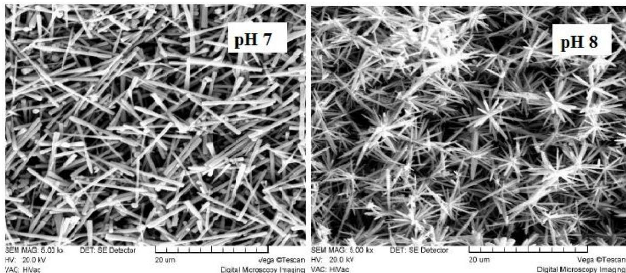
**Fig 1: SEM images of ZnO Nanostructures at pH (Nano wires) and pH 8 (Nano flowers)
