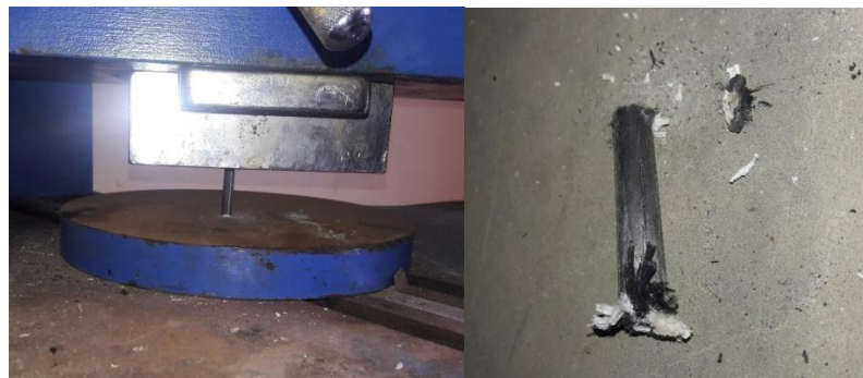
Fig.4:Experimental setup for compression and the failure of the specimen
