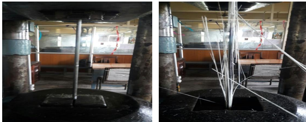
Fig.2: Tensile test and the rupture of hybrid rods
