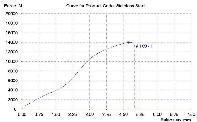
Graph 4.4: Force vs. Extension curve for Sample 2
