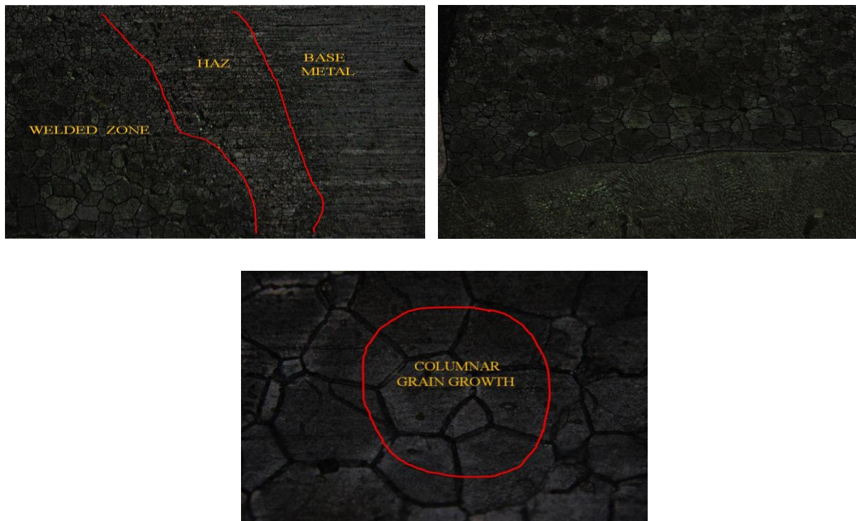
Fig.4.8: Grain growth after Re-crystallization of weld zone
