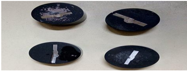
Fig.3.3: Prepared mould to use for microstructure study
