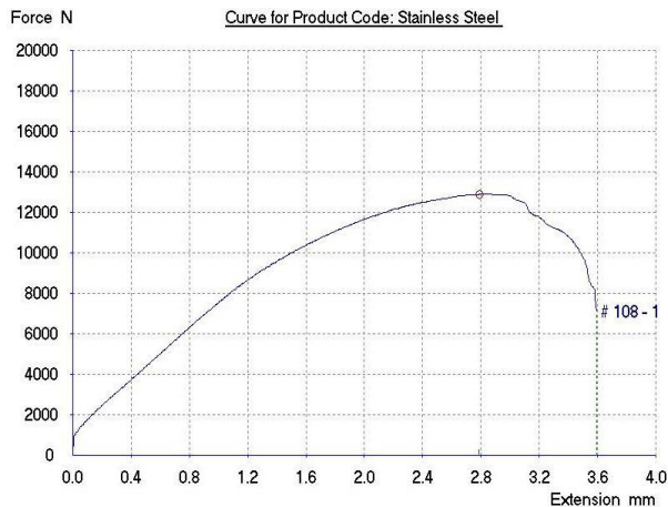
Graph 4.3: Force vs. Extension curve for Sample 1
