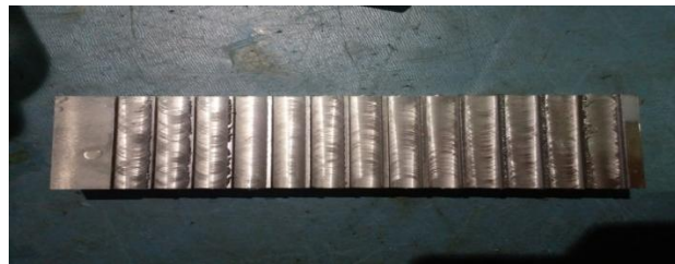
Fig2:- Rectangular plate (207×64×20)mm 3 of EN-31 Alloy steel after slot milling
