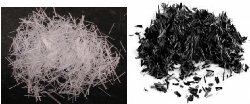
Fig : glass fiber and carbon fiber used for fiber reinforced concrete
