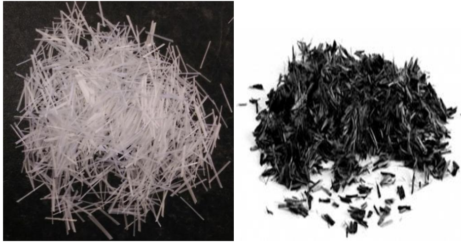
Fig : glass fiber and carbon fiber used for fiber reinforced concrete
