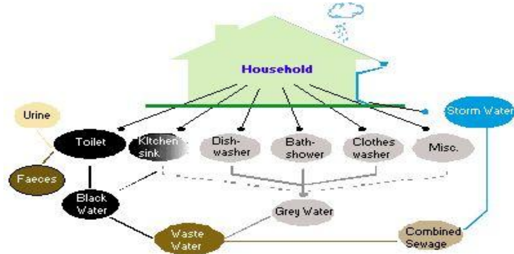
Figure 1: A range of possible sources of household wastewater showing wastewater from toilet, kitchen, bathroom, laundry and others
