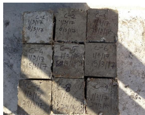
Figure 1 - concrete cubes for testing
