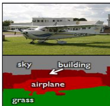
Fig 4: Sample results of simultaneous Object Class Recognition and Segmentation algorithm. Adapted from [5]
