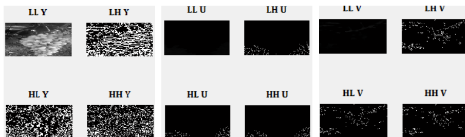
Fig6: Detailed frequency coefficients of YUV components of original image by using DWT
