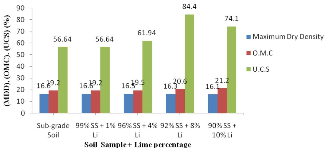
Fig. 3 M.D.D, O.M.C, & U.C.S, of soil sample replaced with different percentages of lime
