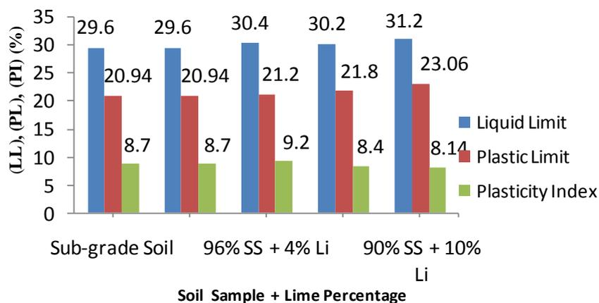
**Fig 2 Soil sample replaced with different percentages of lime. (LL, PL, PI)**
