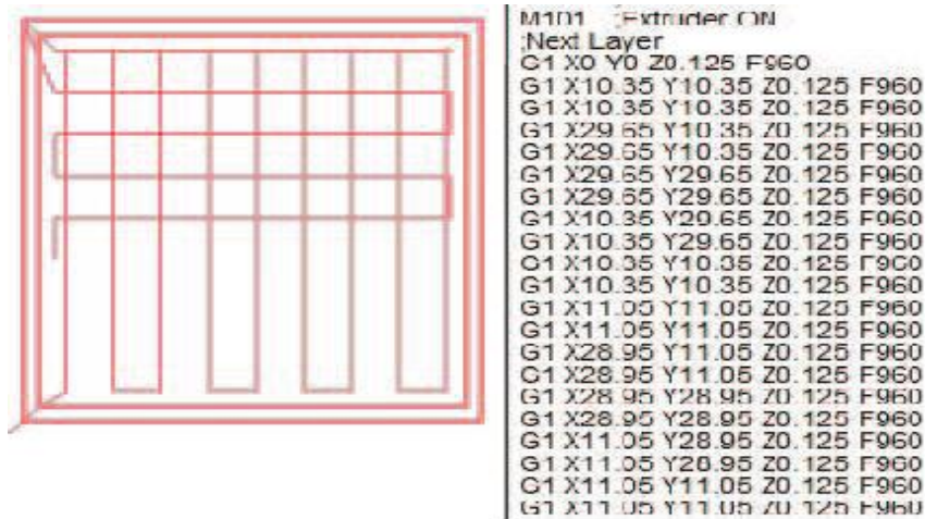
Figure.6. (a) Representation of generated G-Code and (b) Sample resultant G-code of the algorithm.
