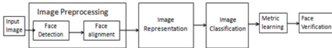
Figure 1: multi-stage Face recognition process
