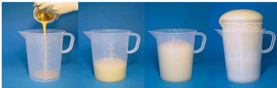
**Figure. 7: Generation of Polyurethane Foam by Hand Mixing**
