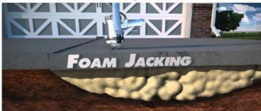
**Figure 6: Raising of Concrete slab by Injection of Polyurethane Foam**
