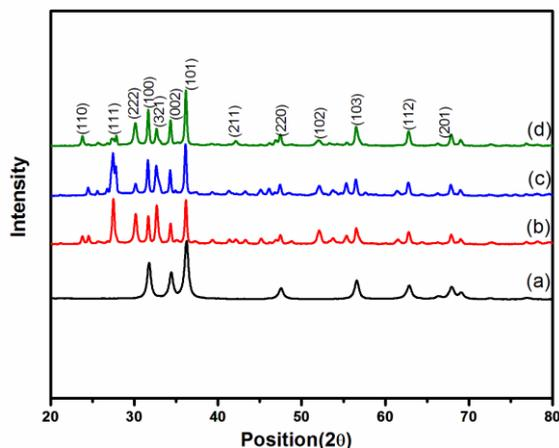
Fig 1.XRD pattern of (a) ZnO (b) Bi<sub>(0.1)</sub>:Zn<sub>(0.9)</sub> O , (c) Bi<sub>(0.15)</sub>:Zn<sub>(0.85)</sub> O (d) Bi<sub>(0.2)</sub>:Zn<sub>(0.8)</sub> O
