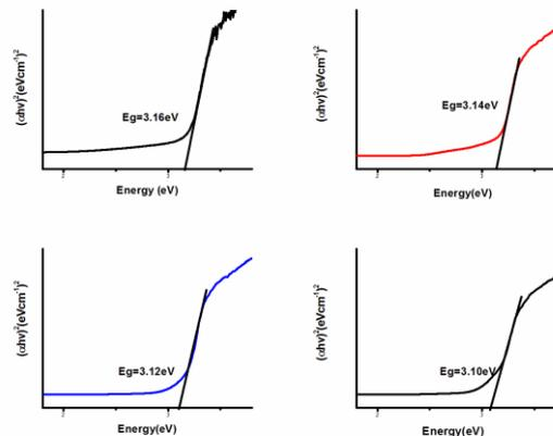
**Fig 5. Tauc plot of (a) ZnO (b) Bi<sub>(0.1)</sub>:Zn<sub>(0.9)</sub>O, (c) Bi<sub>(0.15)</sub>:Zn<sub>(0.85)</sub>O (d) Bi<sub>(0.2)</sub>:Zn<sub>(0.8)</sub>O**
