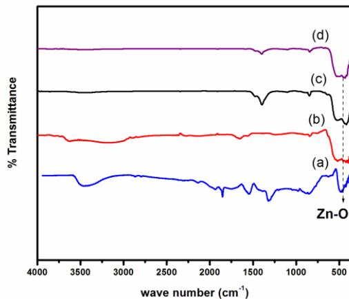
Fig 3. FTIR spectra of (a) ZnO (b) Bi<sub>(0.1)</sub>:Zn<sub>(0.9)</sub>O, (c) Bi<sub>(0.15)</sub>:Zn<sub>(0.85)</sub>O (d) Bi<sub>(0.2)</sub>:Zn<sub>(0.8)</sub>O
