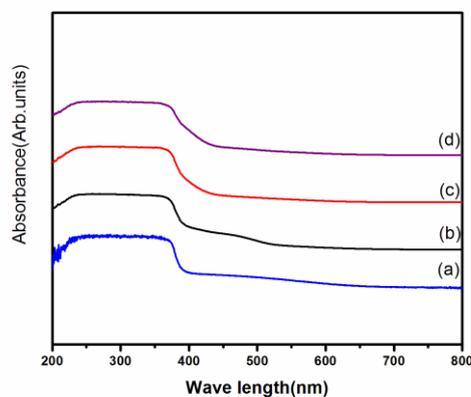
Fig 4. Absorbance s of (a) ZnO (b) Bi<sub>(0.1)</sub>:Zn<sub>(0.9)</sub>O, (c) Bi<sub>(0.15)</sub>:Zn<sub>(0.85)</sub>O (d) Bi<sub>(0.2)</sub>:Zn<sub>(0.8)</sub>O
