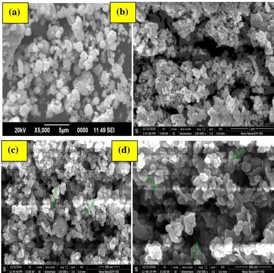
**Fig 2. SEM pattern of (a) ZnO (b) Bi<sub>(0.1)</sub>:Zn<sub>(0.9)</sub> O , (c) Bi<sub>(0.15)</sub>:Zn<sub>(0.85)</sub> O (d) Bi<sub>(0.2)</sub>:Zn<sub>(0.8)</sub> O**
