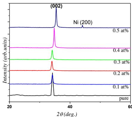
**Figure 1: XRD patterns of pure and Ni doped ZnO thin films**
