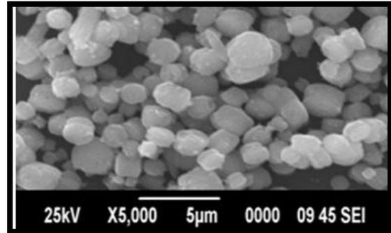
**Figure 2: SEM image of 0.5 at% Ni doped ZnO thin film**
