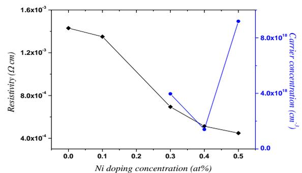
**Figure 3: Variation of electrical resistivity and carrier concentration with Ni doping**
