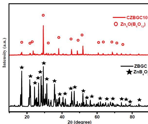
Fig.1. The XRD patterns of (40-x)ZnO-xCuO-60B<sub>2</sub>O<sub>3</sub> (x = 0, 10 mol%) glass ceramics
