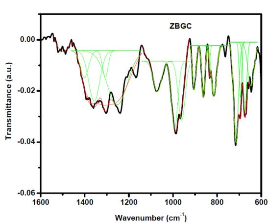
Fig.3.a. The Deconvoluted FT-IR spectra of  $40$  ZnO-  $60\text{B}_2\text{O}_3$  glass ceramics crystallized at  $775^\circ\text{C}$ .
