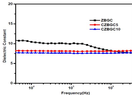
Fig.4.a. The Dielectric studies of  $40$  ZnO-  $60\text{B}_2\text{O}_3$  glass ceramics crystallized at  $775^\circ\text{C}$ .
