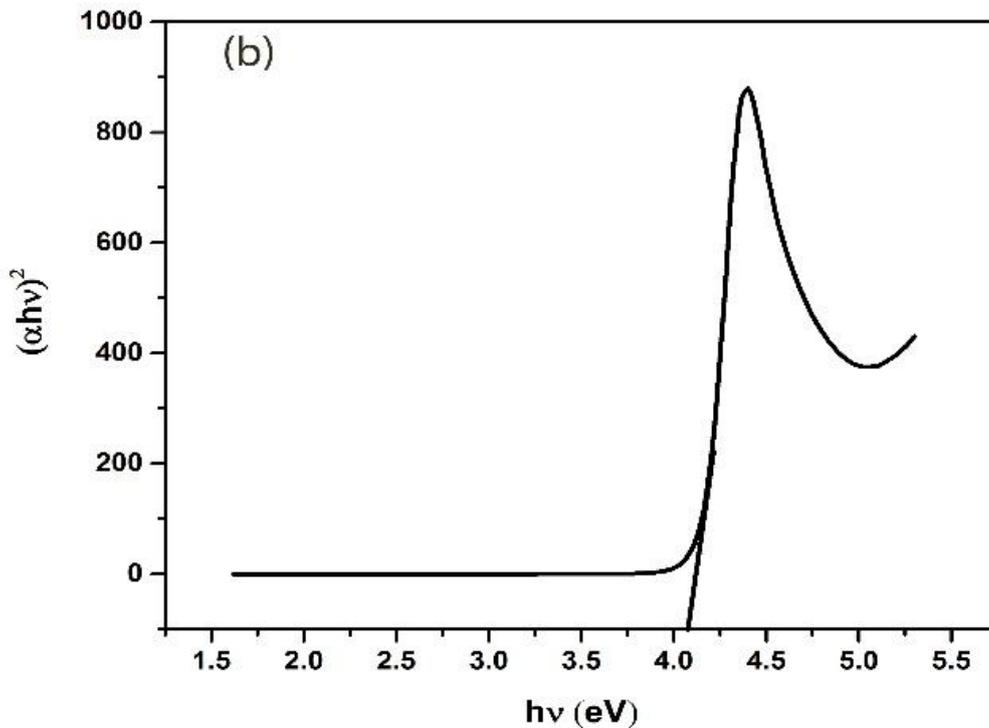
(b)optical band gap of  $Y_2Ti_2O_7$
