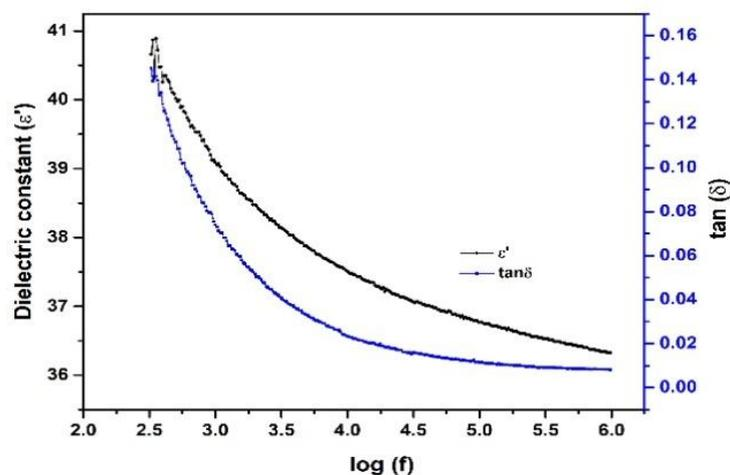
**Fig. 5** Variation of dielectric constant ( $\epsilon'$ ) and loss tangent ( $\tan \delta$ ) for  $Y_2Ti_2O_7$  with frequency
