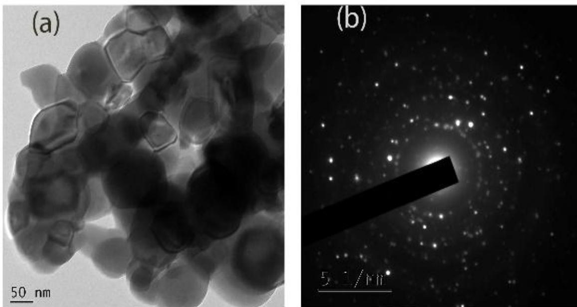
**Fig. 3(a) TEM image and (b) SAED pattern of  $Y_2Ti_2O_7$  nanopowder**
