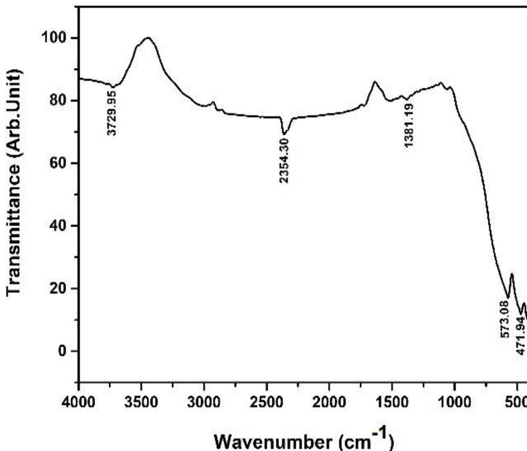
Fig. 2 FT-IR spectra of  $\text{Y}_2\text{Ti}_2\text{O}_7$  sample
