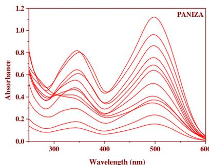
Fig.6 Absorbance spectrum showing photocatalytic degradation of Congo Red using PANIZA
