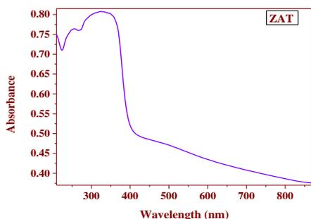
Fig.2 UV/Vis Absorbance spectra of ZAT
