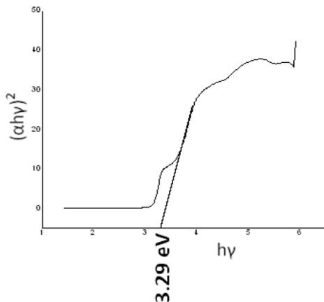
Figure 3A: Optical bandgap calculation of ZnMgO
