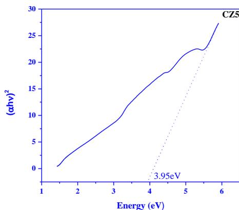
Fig. 3B Optical bandgap calculation of ZnCuO
