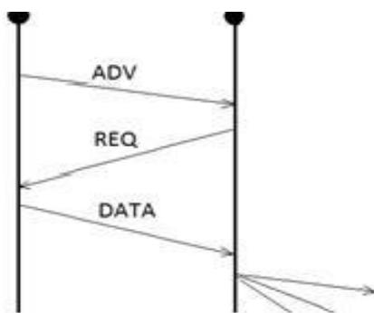
**Fig2. Sensor protocol for information via negotiation (SPIN)**
