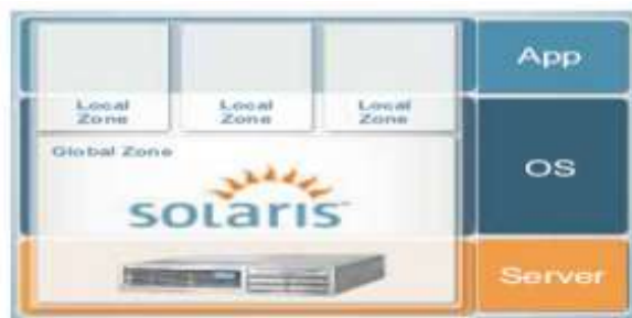
Figure 2: Oracle Solaris Containers enable simple consolidation with isolated, software-defined zones for application and services.
