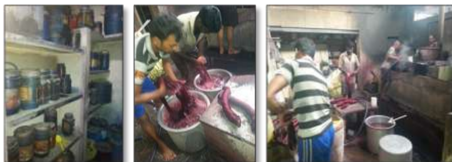
Figure 3.1. (a) Commercial dyes & other chemicals for dyeing fabric (c) Washing dyed fabric (d) Effluent ready to discard (shown with arrow)
