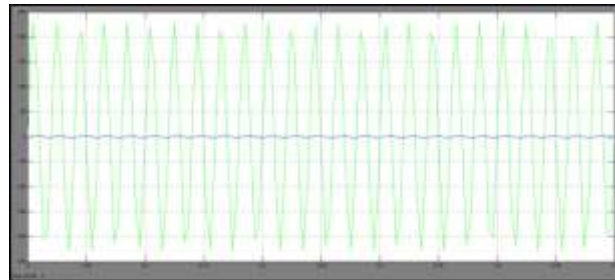
Fig.7: Voltage current waveform without PV solar controller acts as a STATCOM
