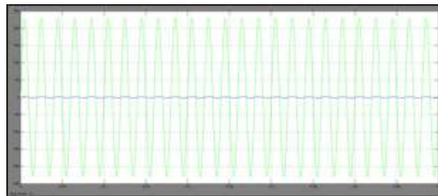
Fig.7: Voltage current waveform without PV solar controller acts as a STATCOM
