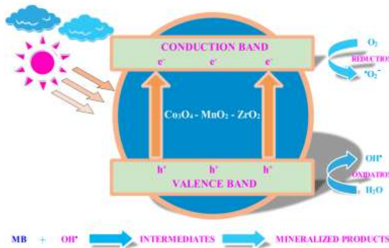
Figure 6. Mechanism for the photocatalytic degradation of MB by \text{Co}_3\text{O}_4 - \text{MnO}_2 - \text{ZrO}_2 NPs
