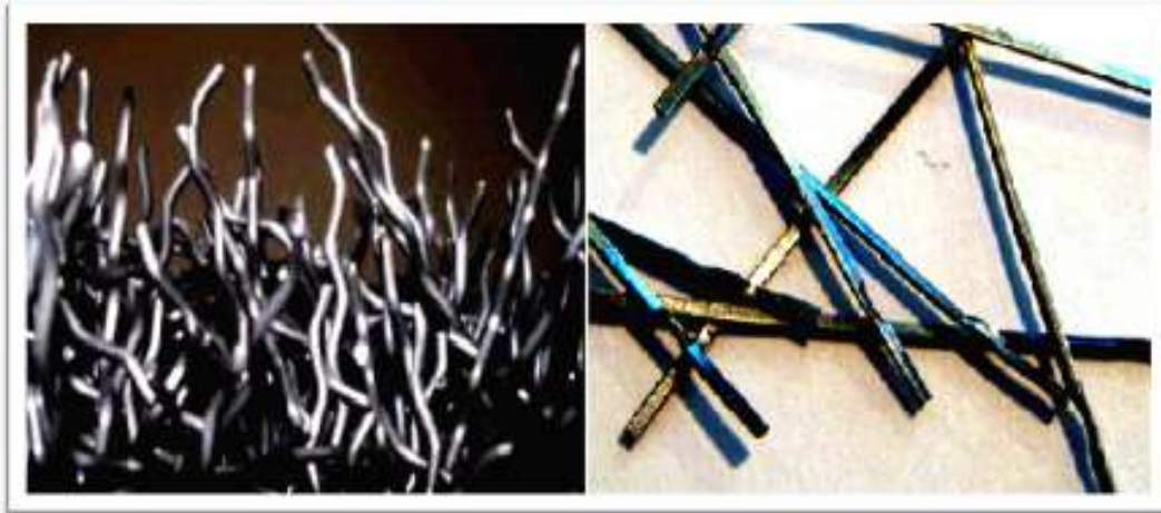
Figure 1.1: Cold-drawn wire fibres
