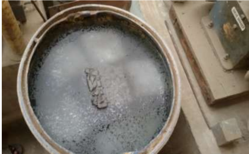
Fig 3: Pervious concrete cube specimens in salt solution
