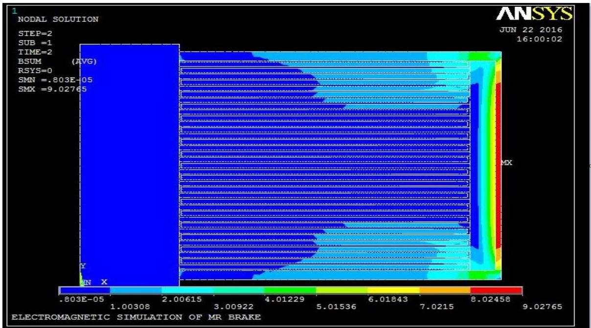
Fig 6. Magnetic flux density by nodal plot.
