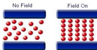
Fig 1. Principle of MR fluid [2]
