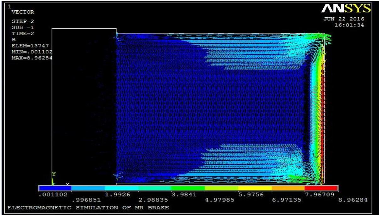
Fig 5. Magnetic flux density by vector plot.
