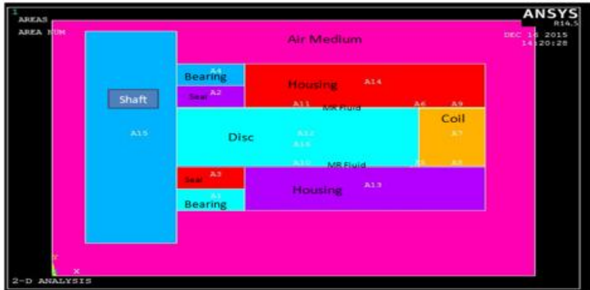
Fig 4. Two dimensional axi-symmetric model of MR brake.
