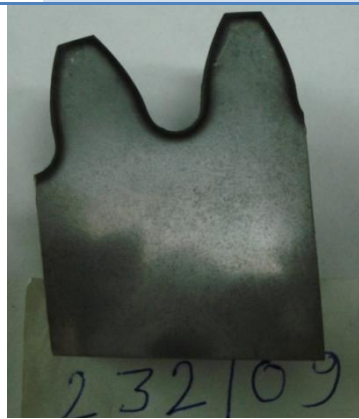
Fig.3 Photograph showing case depth of sample no.232/09/2.
