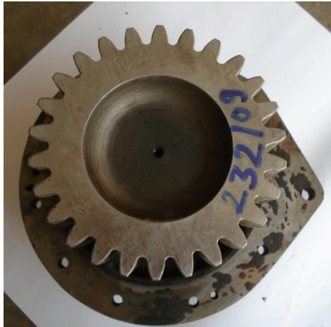
Fig.2 photograph showing auxiliary gear.
