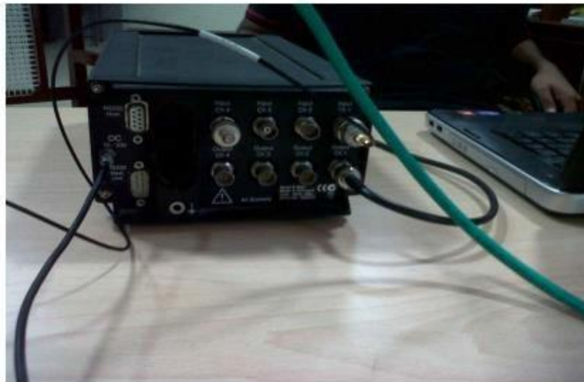
Fig2: Connection of response of accelerometer into the input channel 1 and the connection of BNC Cable, going into the LAN-XI, from the output channel 1
