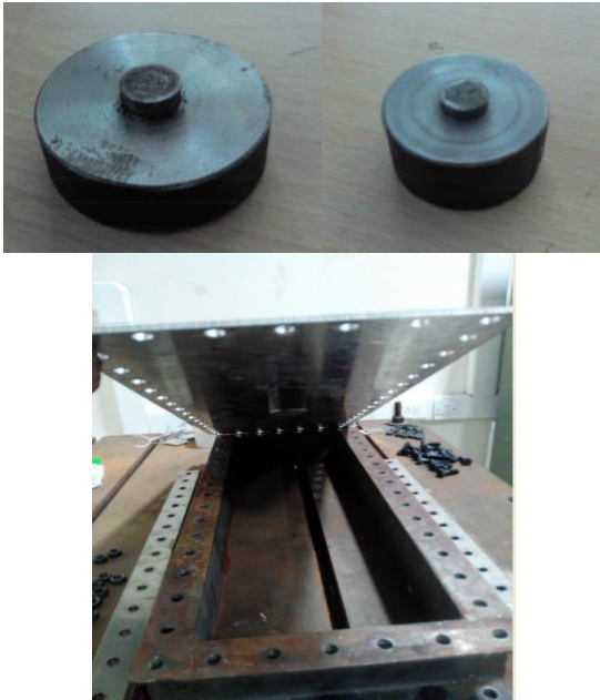
Fig4: Experimental setup demonstrating masses being attached to the Aluminum Plate
