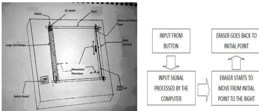
**Fig. class room blackboard erasing machine mechanism and its operating circuit**
