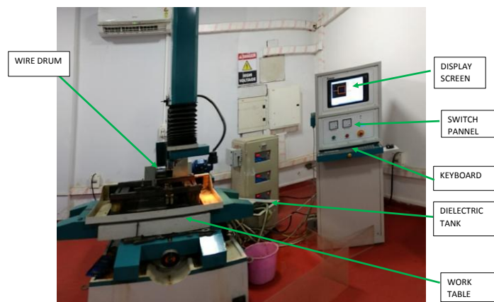
Fig. 2: Schematic diagram of WEDM EZEECUT NXG
