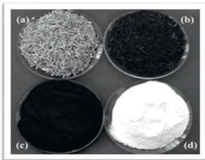
Fig 5.3 (a) Raw Rice Husk (b) Carbonize Rice Husk Ash (c) Grounded Carbonized Rice Husk Ash and (d) Combusted Rice Husk Ash (Grayish White)
