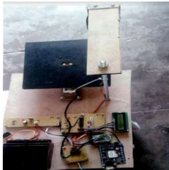
Fig 5: Garbage bin overflow indicator with load cell
