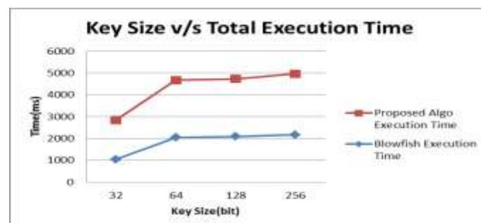
Figure 5: Diagram showing key size v/s Blowfish & Proposed Algorithm's execution time.
