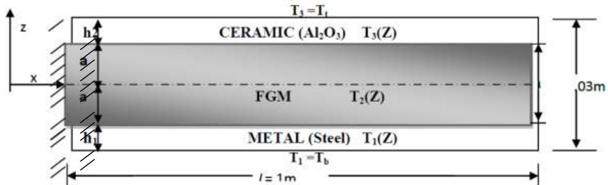
Figure 4.1 Three layer beam with perfect thermal contact at the interface surface
