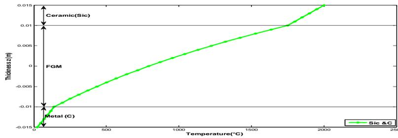
Figure 5.2 (b) Temperature distribution graphs between Sic & C (present work)
