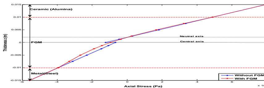
Figure 5.7 (a) Axial stress with FGM & without FGM ( present Work)
