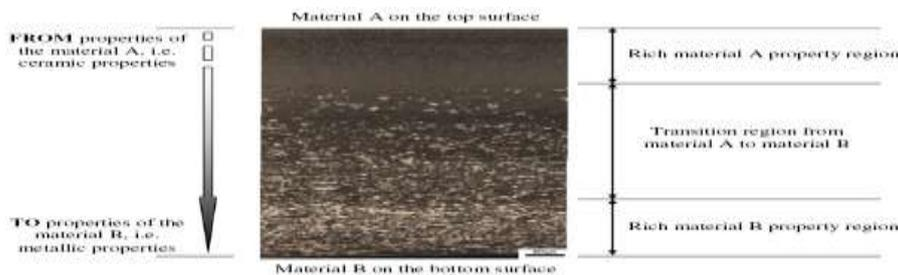
Figure. 3.2a Illustration of the FGM concept by means of microphotography for FGM [1].
