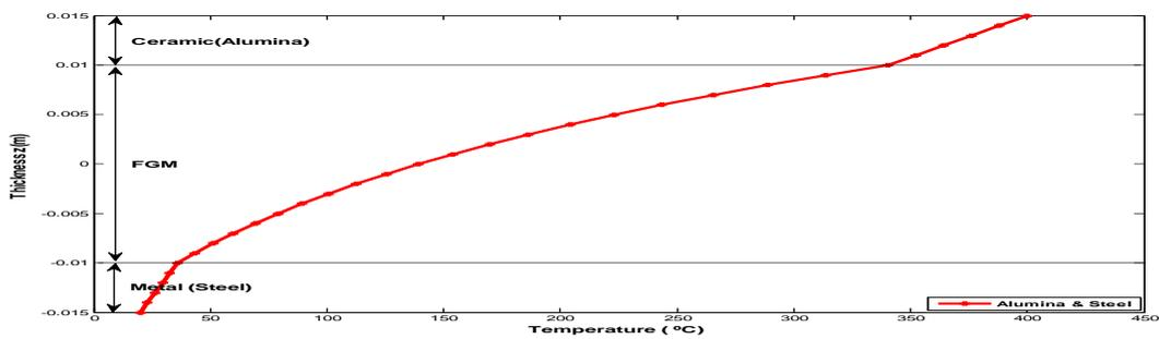
Figure 5.2(a) Temperature distribution graph between Al<sub>2</sub>O<sub>3</sub> & Steel (present work)
