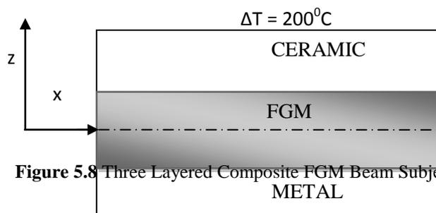
Figure 5.8 Three Layered Composite FGM Beam Subjected to Thermal Loading
