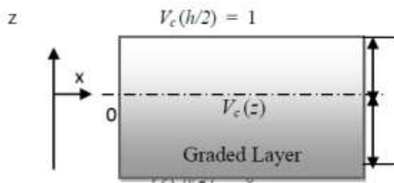
Figure 3.3b Ceramic Volume Fractions Across the FGM Layer
