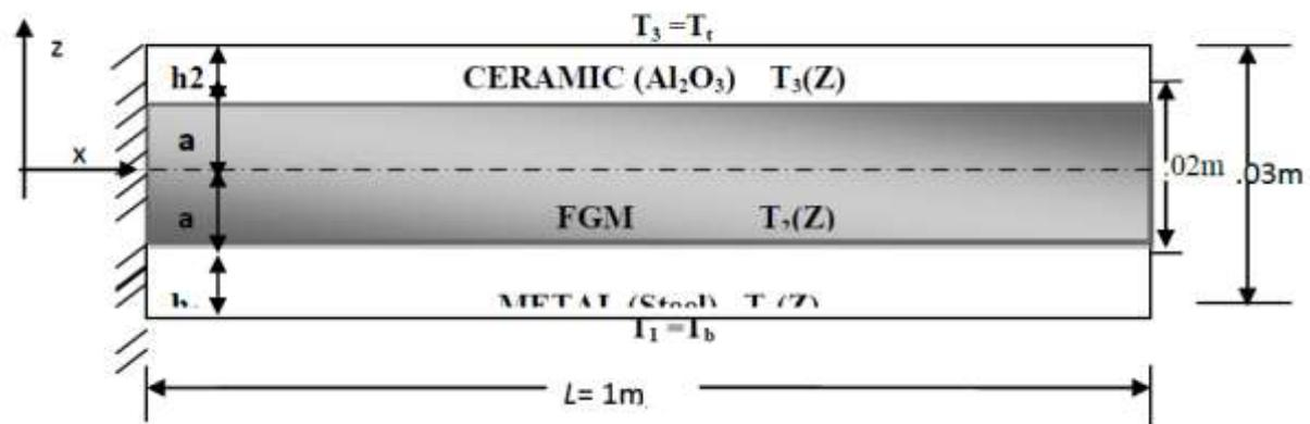
Figure 4.2 Three Layer Composite FGM Beam under Distributed Load
