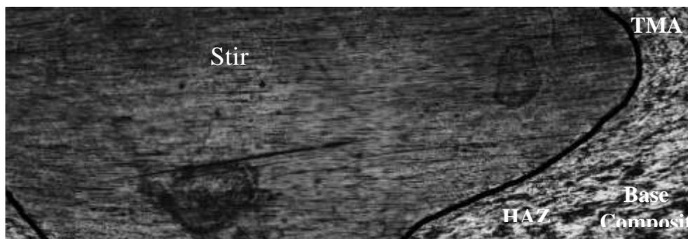
Figure 5: Optical macrograph of the weld cross section showing stir zone, TMAZ, HAZ and base composite
