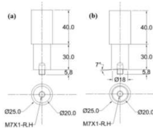
Figure 2: Schematics of the FSW tool used with (a) full flat shoulder, (b) 1mm flat and then 7° concave towards the centre
