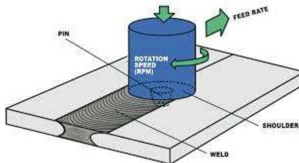
**Figure 1: Friction stir butt welding**
