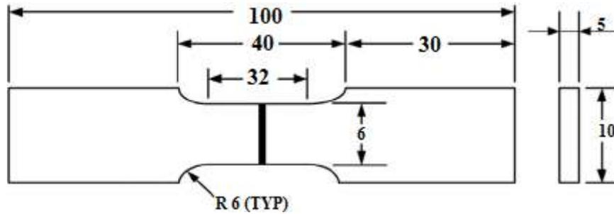
Figure 3: Tensile specimen in accordance with ASTM E8M-04 standard (dimensions in mm)
