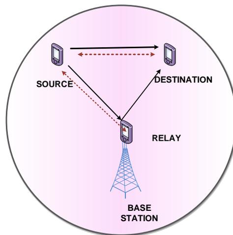
Fig. 3. Relaying device with device controlled link
