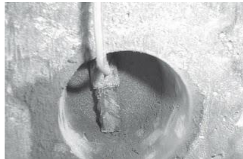
Fig. 4.2 Use of rebar probes in instrumentation
