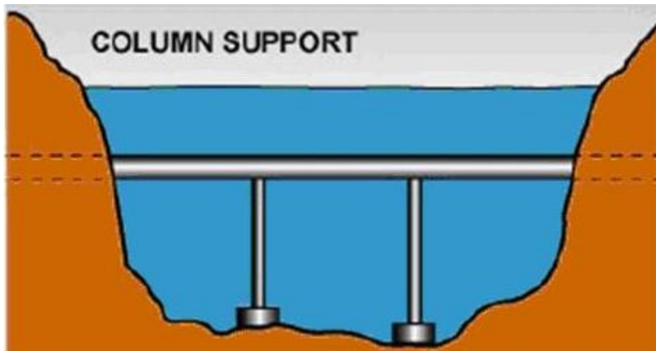
Fig 2.2 SFT supported on columns
