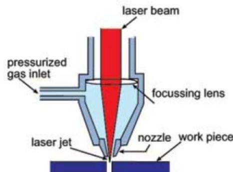
Figure 1: Basic principal of Laser Cutting
