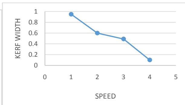
Fig. 6 Kerfwidth vs SPEED
