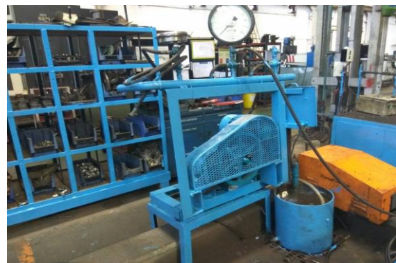
Fig.8. hydro testing pump
