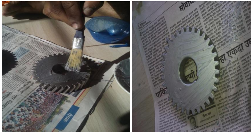
FIG.NO.5.3.3.1 APPLICATION OF ADHESIVE
