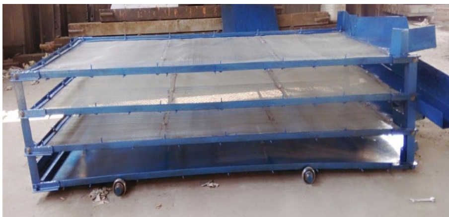
Fig. 3 assembly of four trays, bearings, axles, outlet sections.
