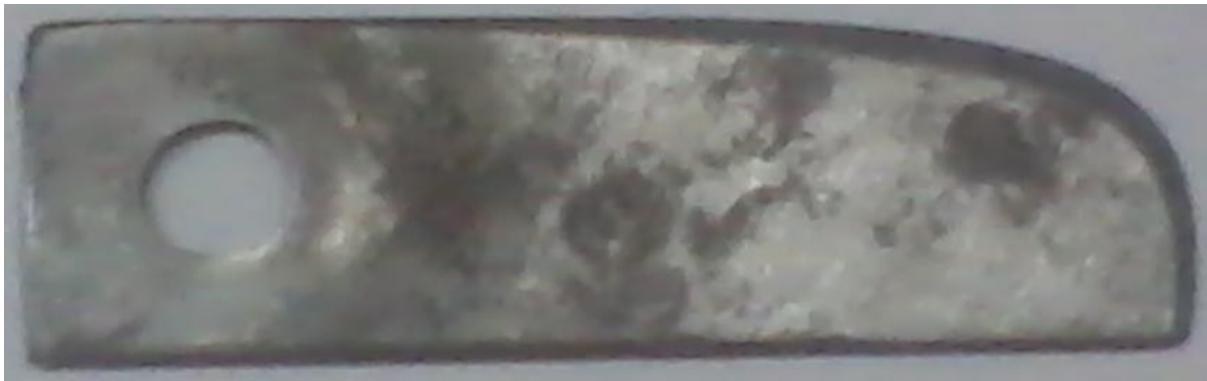
Fig. 13 case hardened and tempered mild steel blade after 15 days of work
