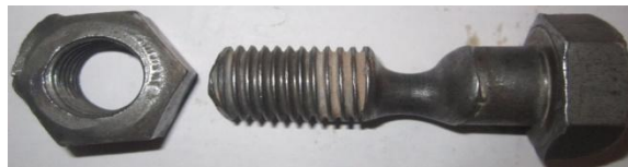
Fig. 7 existing soft bolt after 15 days of work
