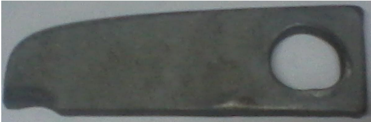
Photo 8.4 Mild steel blade with bush after 15 days of work
