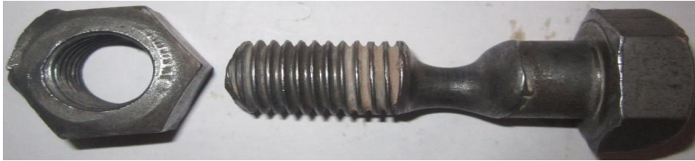
Fig 5 neck formation of bolt
