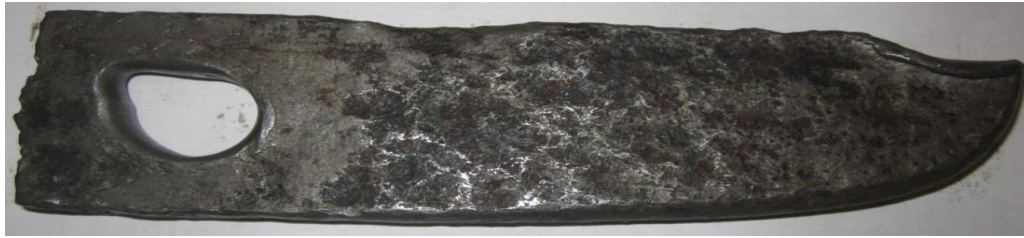
Fig. 4 deformed & weared blade
