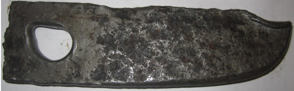
Fig. 12 general mild steel blade after 15 days of work
