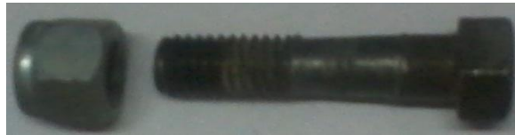
Fig 6 hardened bolt and locknut after 15 days of work
