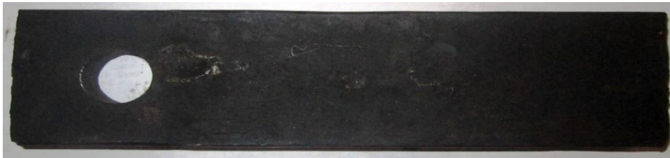
Fig. 8 case hardened and tempered mild steel blade
