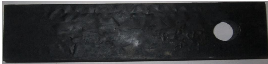
Fig 9 hardened and tempered EN31 blade
