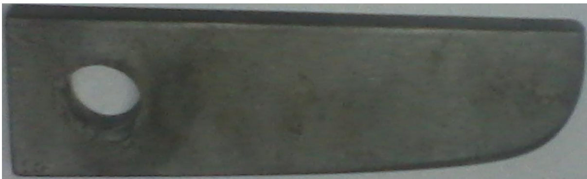
Fig. 14 hardened and tempered en31 blade after 15 days of work
