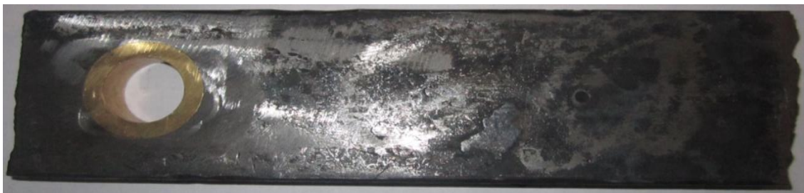
Fig. 10 general mild steel blade with brass bush
