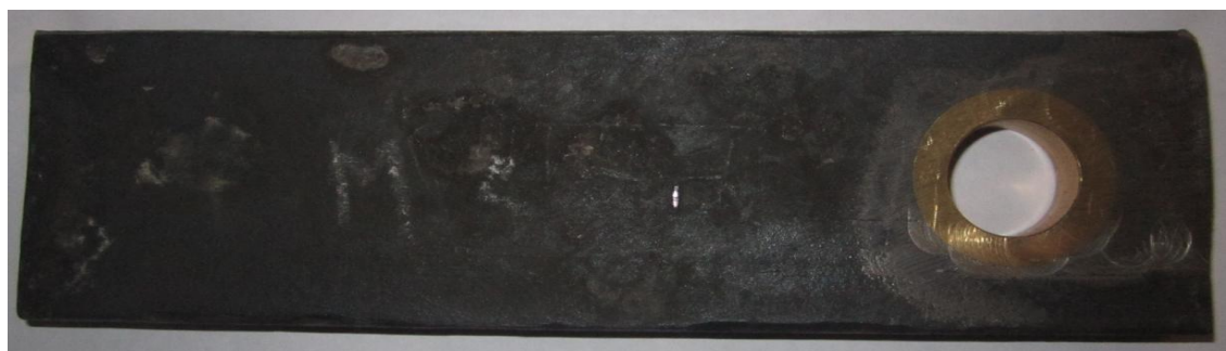
Fig. 11 hardened mild steel blade with brass bush
